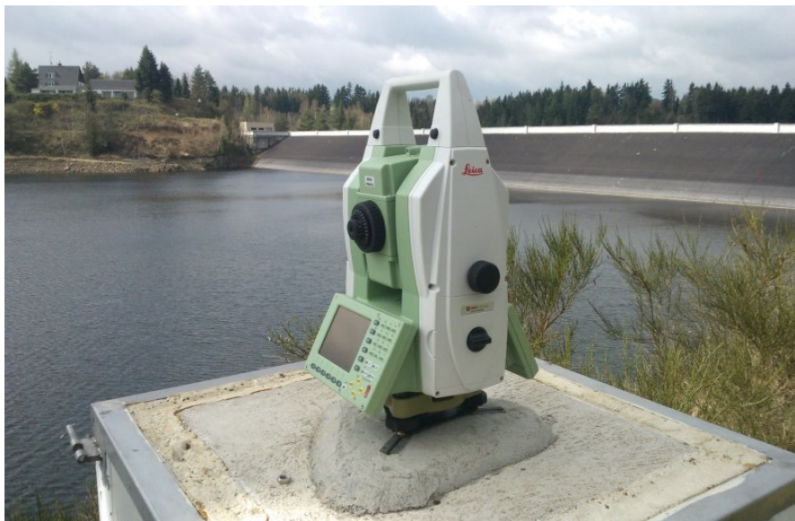
Fig. 1 Leica TM30, Stanovice dam
